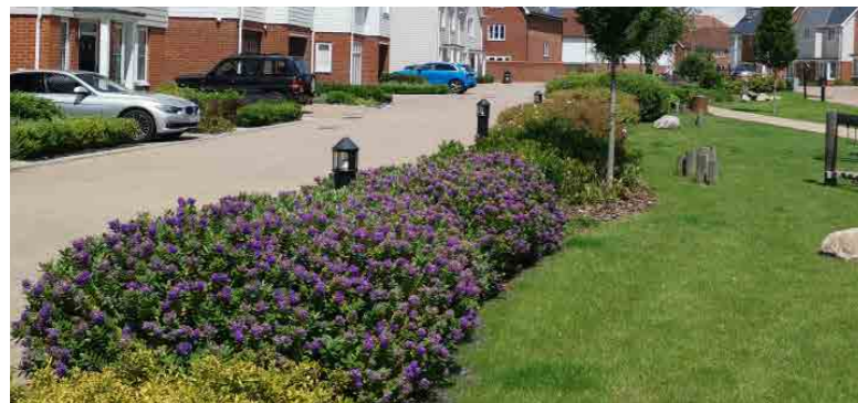
Shrub planting used along sections of the road to stop parking on the greenway.
