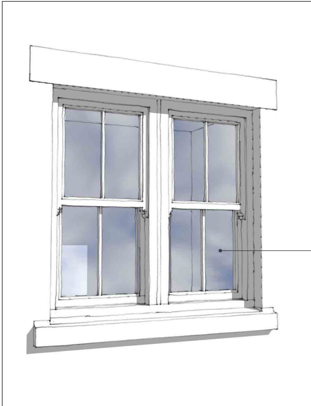
PVCU Sliding Sash Windows with Off White or Grey Green Foil
