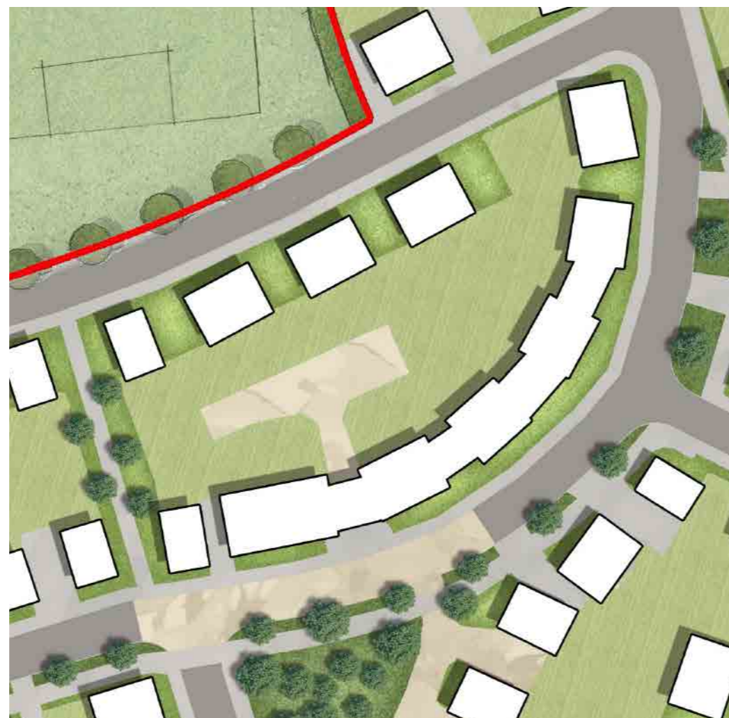
Typical block design designed to maintain minimum back to back distances to prevent overlooking.
